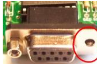
Figure Cb - Screw connector removed
