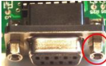
Figure Ca – Screw connector in place
